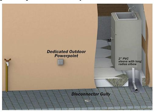
Stage 2: Installing the G-Flow system & the irrigation components (Preferably before paving work)
